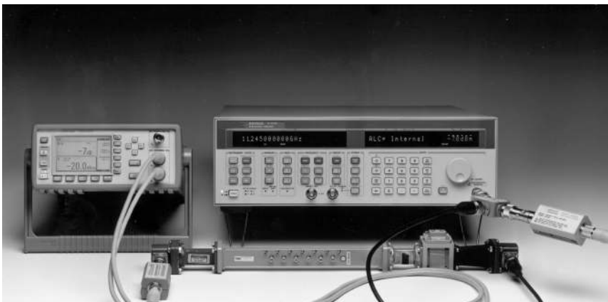
Figure 4-10. E4419B dual-channel power meter measures insertion loss of a 11.245 GHz waveguide bandpass filter, using the meter’s power ratio mode, plus a sweeper and power splitter. Keysight’s 90 dB dynamic-range sensors are ideal for such high-attenuation measurements.
